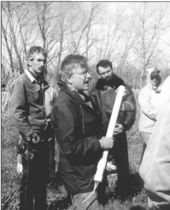
Don Huggins, Kansas Biological Survey, explains a groundwater sampler and the testing they are conducting on the Bruce Spare farm to farmers.
